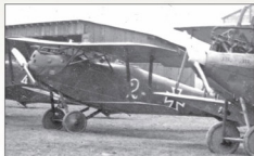
Hannover Cl.II 9295/17 was from the 1st production order for 200 aircraft (numbers 9200/17 to 9399/17) placed in August 1917. Aircraft from this production batch were delivered without the additional tailplane bracing struts (D9) but many had them retrofitted when they became available (and if the aircraft lasted long enough).
