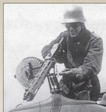
LMG 14 Parabellum fitted to an unidentified Hannover CL.II, CL.III or CL.IIIa. Note the unpainted aluminium(?) magazine and the empty belt protruding from the side of the gun. Although obviously posed, this photo shows both the pilot and observer wearing steel helmets which could be worn during dangerous ground attack operations.
