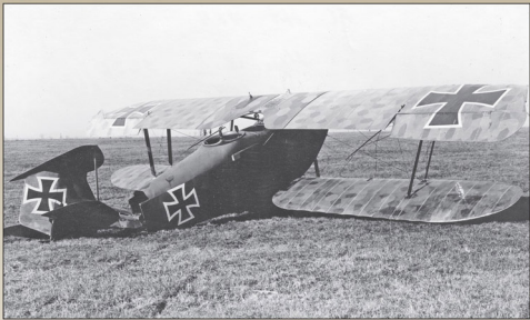
The very dark fuselage of FA 46b Hannover Cl.II 9290/17 (wn 645) has broken its back after what appears to be a rather heavy landing. Note the pristine 5 colour lozenge covered wings, ailerons and rudder. The starboard bottom wing appears to have CDL rib tapes while the others appear to have rib tapes cut from lozenge material.
