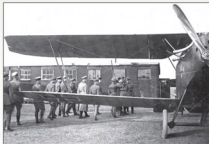
Hannover Cl.II 9295/17 was from the 1st production order for 200 aircraft (numbers 9200/17 to 9399/17) placed in August 1917. Aircraft from this production batch were delivered without the additional tailplane bracing struts (D9) but many had them retrofitted when they became available (and if the aircraft lasted long enough).
