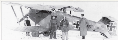
The unidentified crew of this FA 7 (Fliegerabteilung 7) Hannover CL.II 9339/17 prepare for a chilly flight during the winter of 1917-18. Note the makeshift 'safety bar' added above the center section cut out to prevent the gunner from shooting the propeller and, perhaps more importantly, the gravity fuel tank. An Oigee, or possibly a captured Aldis, sight has been fixed to the Parabelium LMG 14 machine gun. The fuselage number '5' could be red or black and we have supplied both for you to choose from. Wide bands of unconfirmed camouflage colours have been sprayed over the fuselage and the green and Prussian blue illustrated here are what we consider quite likely but the final decision is yours. No weight table is visible under the pilot's cockpit. A small bullet hole patch is visible between the fuselage eisernkreuz and FA 7 arrow marking.
